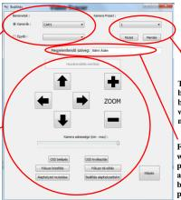
The set positions is stored by the camera. With these buttons it is possible to write and read the camera memory.
