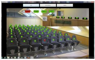
The image above shows a real scene. The small round buttons mark camera positions, which are ordered to chairs. The red button shows that participant, who is speaking. The oblong video source selector buttons can be seen on the top of the screen. Use these buttons to choose the displays and the recording sources.
